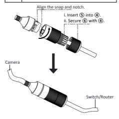
Figure 2-7 Water-proof Accessory Installation
