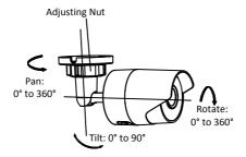
Figure 2-5 3-axis Adjustment
